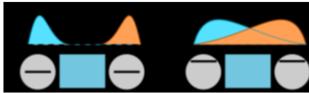
Figure 1: Sketch of a minimal Kitaev chain formed by two QDs coupled via a superconducting segment, hosting well-localized (a), and overlapping MBSs (b).
